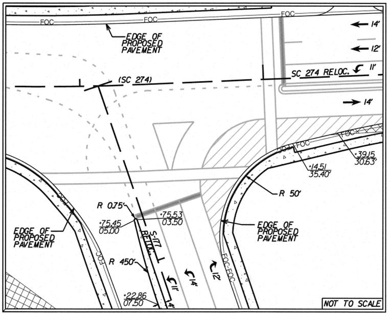
RELOCATE S-177 CENTERLINE BETWEEN STA.10+00.00 AND STA.11+10.80
